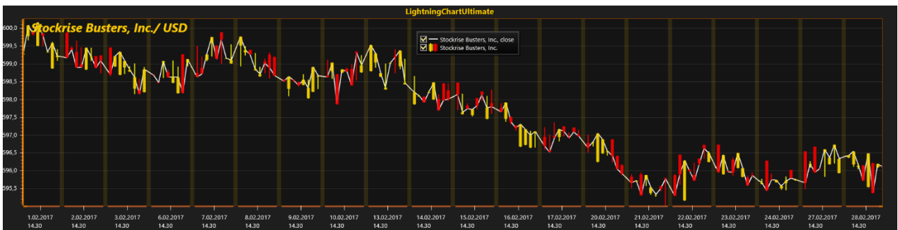
Figure 6-36. ScaleBreaks applied to exclude non-active trading hours. More screen space is available for essential data. Style = Fill, Gap = 10. PointLineSeries jumping from Close-to-Close values, PointLineSeries.ContinuousOverScaleBreak = True.
