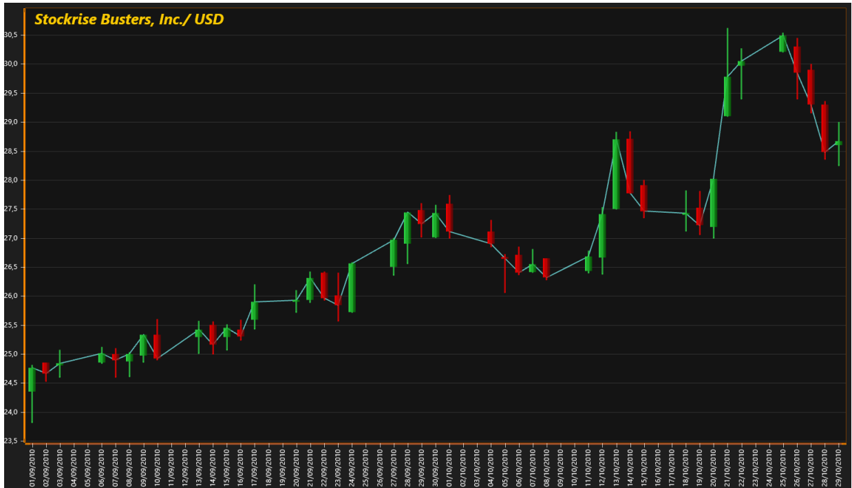
Figure 6-60. One StockSeries with Style = CandleStick. Light blue line is a PointLineSeries in the background going through all Close values.
