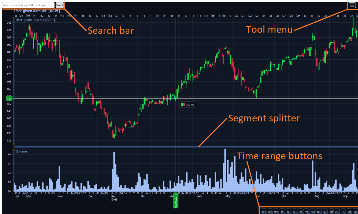
Figure 18-4. TradingChart's main user interface components, all of which can be hidden by disabling the respective property.
