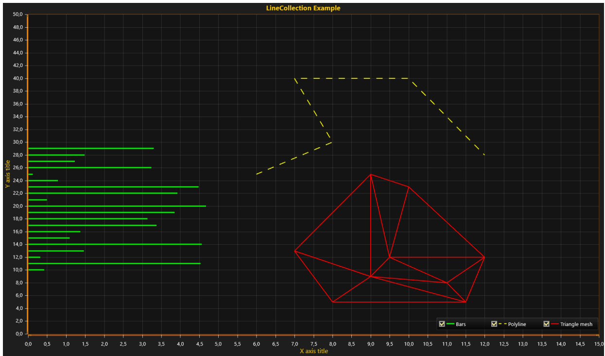
Figure 6-65. Three LineCollections in use. Green acts as very rapidly rendering bars, yellow as a polyline, and red as an arbitrary triangle wireframe mesh.
